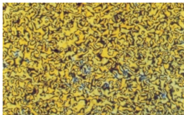
Figure 1. Optical textures of 5 . Photomicroscopic images of the mesophase were obtained with a polarizing microscope (Leitz DMRXP equipped with a Mettler FP82HT hot stage) on cooling from the isotropic liquid at 25 °C (crossed polarizer, magnification \times 100 )
